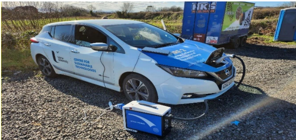
Figure 8 - Image showing testing of V2L technology using Nissan Leaf as part of previous case study.
